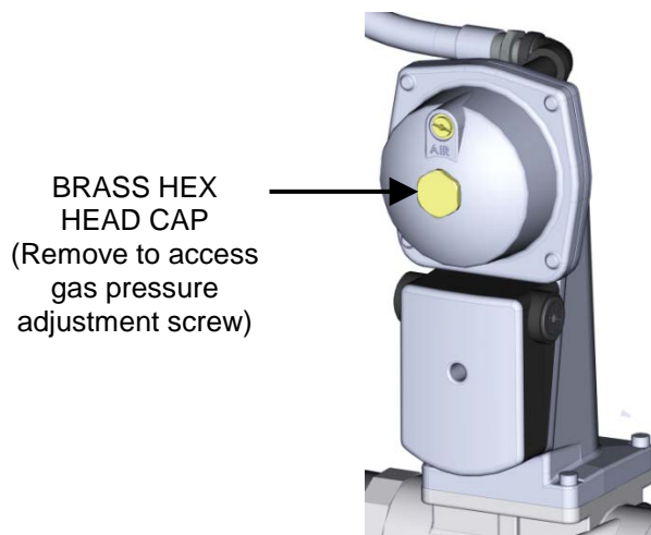
Figure 4-4. Gas Pressure Adjustment Screw Location
