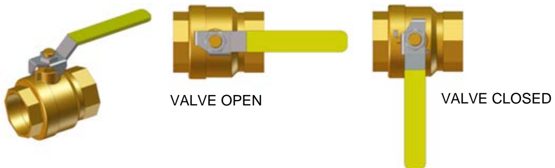
Figure 1-1. Manual Gas Shutoff Valve
