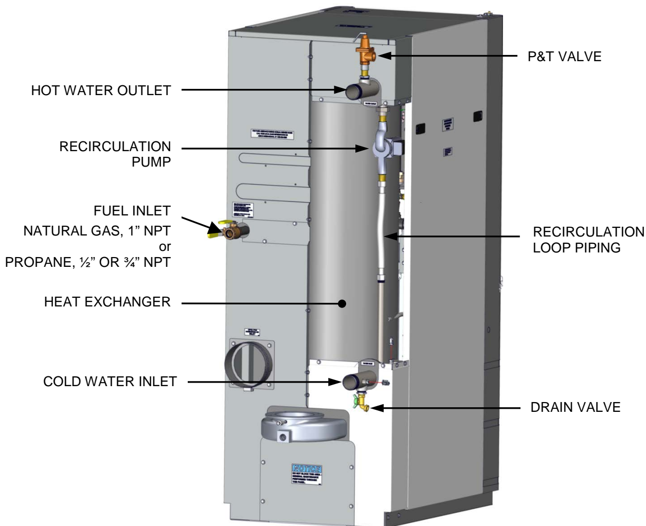
REAR VIEW – REAR PANEL & EXHAUST VENT REMOVED
