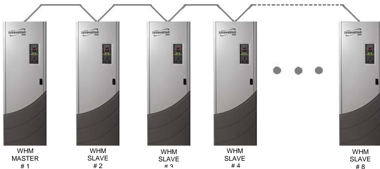
Figure 8-3. Typical Daisy-Chain Modbus/RS485 Network
