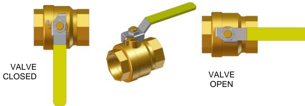
Figure 1-1: Manual Gas Shutoff Valve
