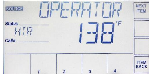
All heaters are factory set to 120F. if replacing a PIM module in the field, this must be adjusted.
